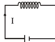
If direct current is connected across inductor current increases with time and transformer is also inductor. So, current can increase to large value and transfer can burn.]
