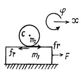
But at the moment  $t = t_0$ , when pure rolling starts  $v_c = \omega R$
