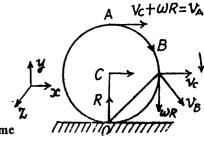
As point O is the instantaneous centre of rotation of the ball at the moment shown in Fig. so,  $\vec{v_0} = 0$ ,
