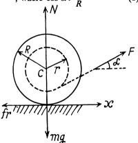
Note that at  $\cos \alpha = r/R$ , there is no rolling and for  $\cos \alpha < r/R$ ,  $w_{cx} < 0$ , i.e. the spool will move towards negative x-axis and rotate in anticlockwise sense.
