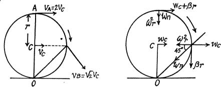
As, an arbitrary point of the cylinder follows a curve, its normal acceleration and radius of curvature are related by the well known equation
