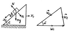
1.82 To analyse the kinematic relations between the bodies, sketch the force diagram of each body as shown in the figure.
