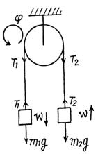
1.247 As the system  $(m + m_1 + m_2)$  is under constant forces, the acceleration of body  $m_1$  an  $m_2$  is constant. In addition to it the velocities and accelerations of bodies  $m_1$  and  $m_2$  are equal in magnitude (say  $\nu$  and  $m_2$ ) because the length of the thread is constant.
