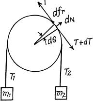
(b) When  $\frac{m_2}{m_1} = \eta$ , which is greater than  $\eta_0$ , the blocks will move with same value of acceleration. (say w) and clearly  $m_2$  moves downward. From Newton's second law in projection form (downward for  $m_2$  and upward for  $m_1$ ) we get:
