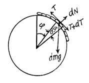
1.108 In the problem, we require the velocity of the body, realtive to the sphere, which itself moves with an acceleration  $w_0$  in horizontal direction (say towards left). Hence it is advisible to solve the problem in the frame of sphere (non-inertial frame).
