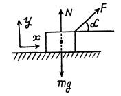
$$m\int_{0}^{x} dv_{x} = a \cos \alpha \int_{0}^{x} t dt \quad \text{(using Eq. 1)}$$
