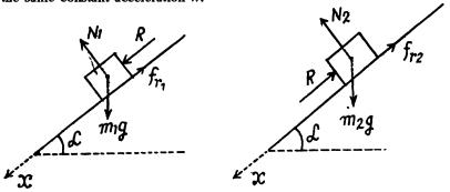
Newton's second law of motion in projection form along x-axis for the blocks gives:
