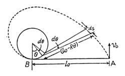
It should be clearly understood that the only uncompensated force acting on the disc A in this case is the tension T, of the thread. It is easy to see that there is no point here, relative to which the moment of force T is invarible in the process of motion. Hence conservation of angular momentum is not applicable here.
