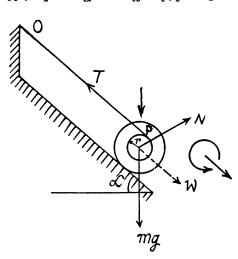
1.256 Let us sketch the force diagram for solid cylinder and apply Newton's second law in projection form along x and y axes (Fig.):
