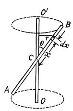
1.270 Let us consider the system in a frame rotating with the rod. In this frame, the rod is at rest and experiences not only the gravitational force  $m \ g$  and the reaction force R, but also the centrifugal force  $F_{cf}$ .
