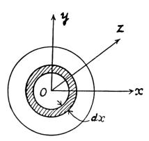
1.241 For simplicity let us use a mathematical trick. We consider the portion of the given disc as the superposition of two complete discs (without holes), one of positive density and radius R and other of negative density but of same magnitude and radius R/2.
