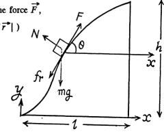
1.122 Let s be the distance covered by the disc along the incline, from the Eq. of increment of M.E. of the disc in the field of gravity:  $\Delta T + \Delta U = A_{fr}$
