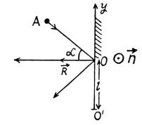
Here,  $\Delta \vec{M} = \vec{r}_{oo'} \times \Delta \vec{p} = 2 \, mv \, l \cos \alpha \, \hat{n}$  and directed normally emerging from the plane of figure
