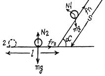
1.123 Let x be the compression in the spring when the bar  $m_2$  is about to shift. Therefore at this moment spring force on  $m_2$  is equal to the limiting friction between the bar  $m_2$  and horizontal floor. Hence
