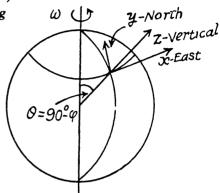
1.112 The disc exerts three forces which are mutually perpendicular. They are the reaction of the weight, mg, vertically upward, the Coriolis force 2mv'  $\omega$  perpendicular to the plane of the vertical and along the diameter, and  $m\omega^2 r$  outward along the diameter. The resultant force is,
